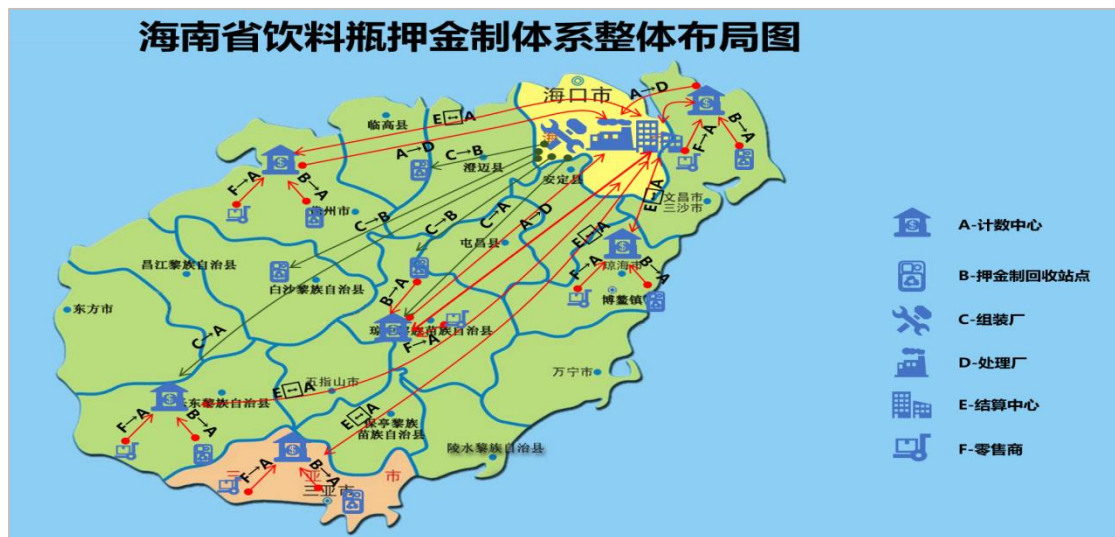
Fig. 5 Smart deposit system layout for beverage bottle collection in Hainan
